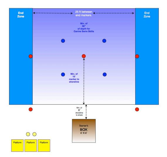
**SQUARE LOOPING** patterns. There shall be four navigation markers, set ten feet apart around the center distance marker. The navigation markers shall appear to be the corners of a square shape.
